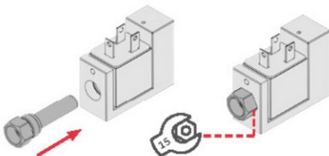
3. Insert the micrometric adjustment and with a 13mm wrench screw it into the valve body;
