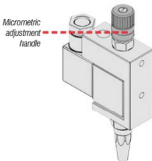
**A. Turn counter-clockwise to increase the needle travel therefore the dispensed fluid quantity.**
