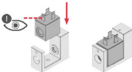
2. Insert the guide sleeve through the valve body and the coil, then screw it with a 15mm wrench;
