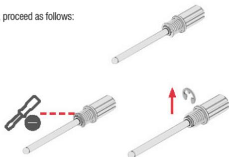
2. Pull out the spring from the needle;
