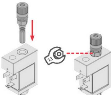
4. Insert the needle inside the guide sleeve;
