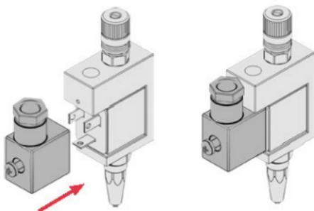
7. Finally screw the coil connector screw.
