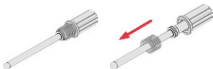
3. Finally pull out the washer.
