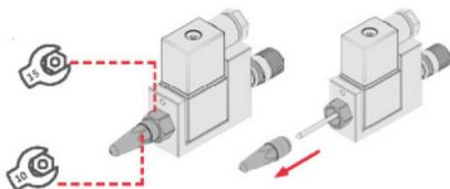
After removing the nozzle, to clean it:
