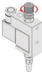
2. Unscrew the nozzle with a 10mm wrench by holding the guide sleeve with a 15mm wrench;
