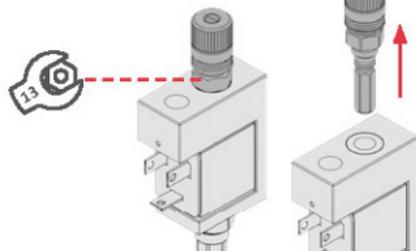
4. Check the wear of the micrometric adjustment O-ring and if it is necessary, replace it. Always grease\* the new O-rings before assembling them;
