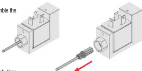
7. Unscrew the guide sleeve with a 15mm wrench, then pull it out from the valve, being careful not to drop the coil on the ground because it will be free to move;
