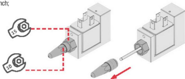
6. Pull out the needle using fingers (to disassemble the needle see section 6.5 - Needle disassembly);
