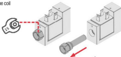
8. Remove the coil from the valve body;
