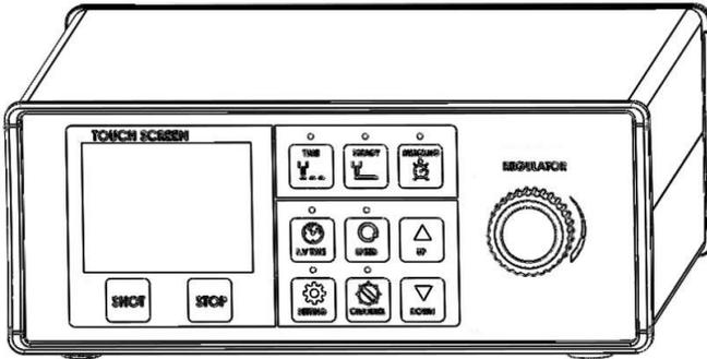
The PCP volumetric pumps allow dispensing fluids with various types of viscosity with maximum repeatability. The Controller allows to set all the dispensing parameters.
