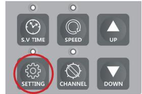
This menu allows you to select some operating parameters of the pump and to check the status of the interface between the pump and the PLC; when the SETTING button is pressed for at least 2 seconds, the screen shown here appears.
