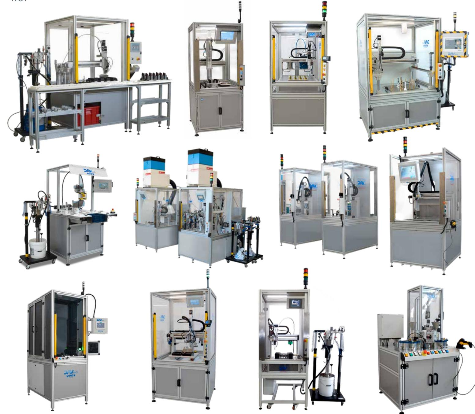
**2K Dispensing stations** All our applications are based on volumetric proportioning systems managed by controllers and/or PLCs, this allows the process to be controlled with highest precision and to guarantee reliability.
