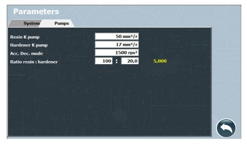
• RESIN (A)/HARDENER (B) K PUMP: indicates the volume of product dispensed with each complete rotation of the pump. The table below shows the actual indicative displacements of each pump model.
