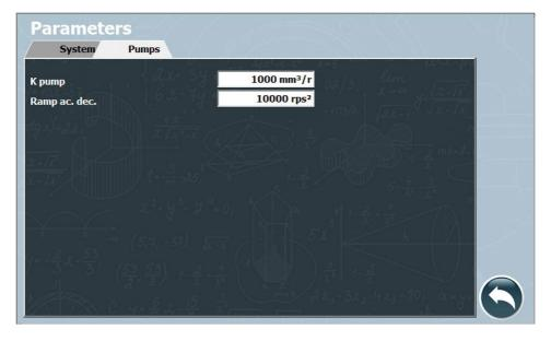
• **K PUMP:** indicates the volume of product dispensed with each complete rotation of the pump. The table below shows the actual indicative displacements of each pump model.
