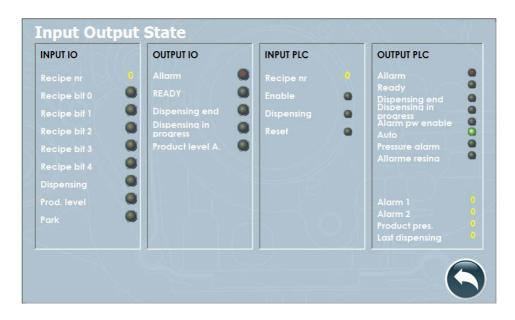
On this page you can view in real time all the states of the controller inputs and outputs.
